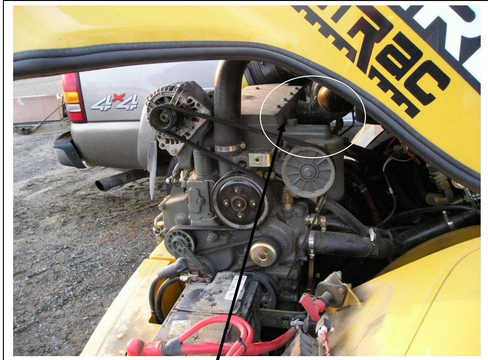
Compressor mount area.
